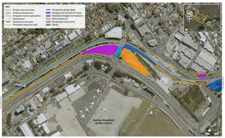
Figure 7.7b Project site – Construction footprint and proposed work areas
