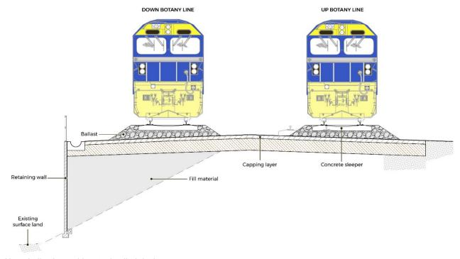
Figure 6.5 Indicative track formation with retaining wall
