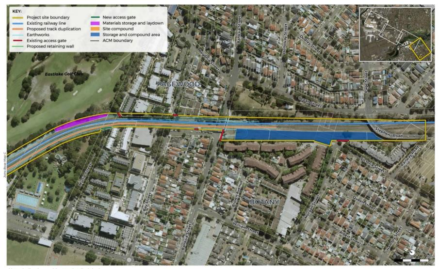
Figure 7.7d Project site – Construction footprint and proposed work areas
