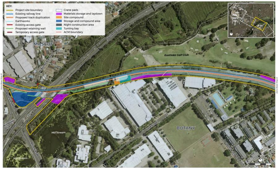
Figure 7.7c Project site – Construction footprint and proposed work areas
