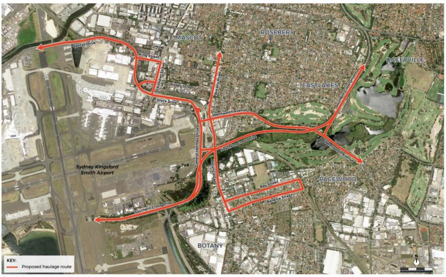
Figure 7.9 Construction vehicle routes – heavy vehicles
