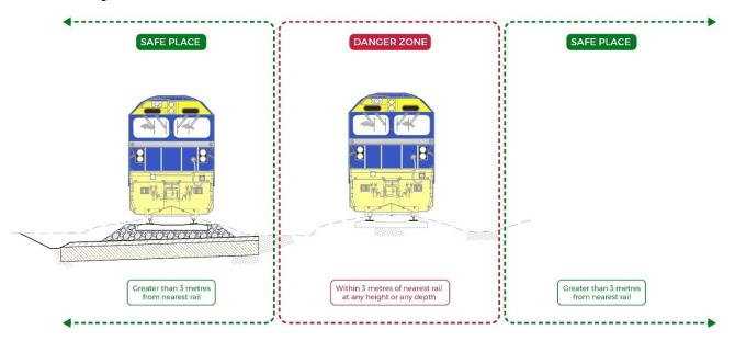
Note: The above diagram illustrates the potential danger zone where the rail track on the right is the live/active rail corridor while the track on the left hand side is being constructed.
