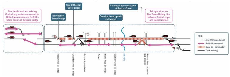
Figure 7.6 Indicative construction staging – Stage 2B: Construct new O'Riordan Street and Robey Street bridges
