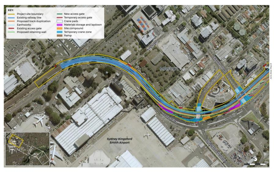
Figure 7.7a Project site – Construction footprint and proposed work areas
