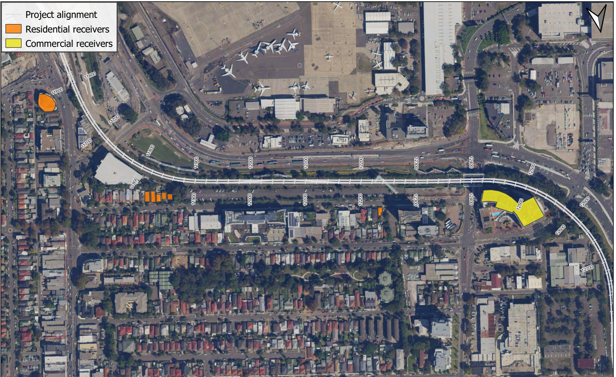
Year 2024 Build Scenario - With EPA Licencing and Lubrication Sensitive Receivers Exceeding Noise Criteria
