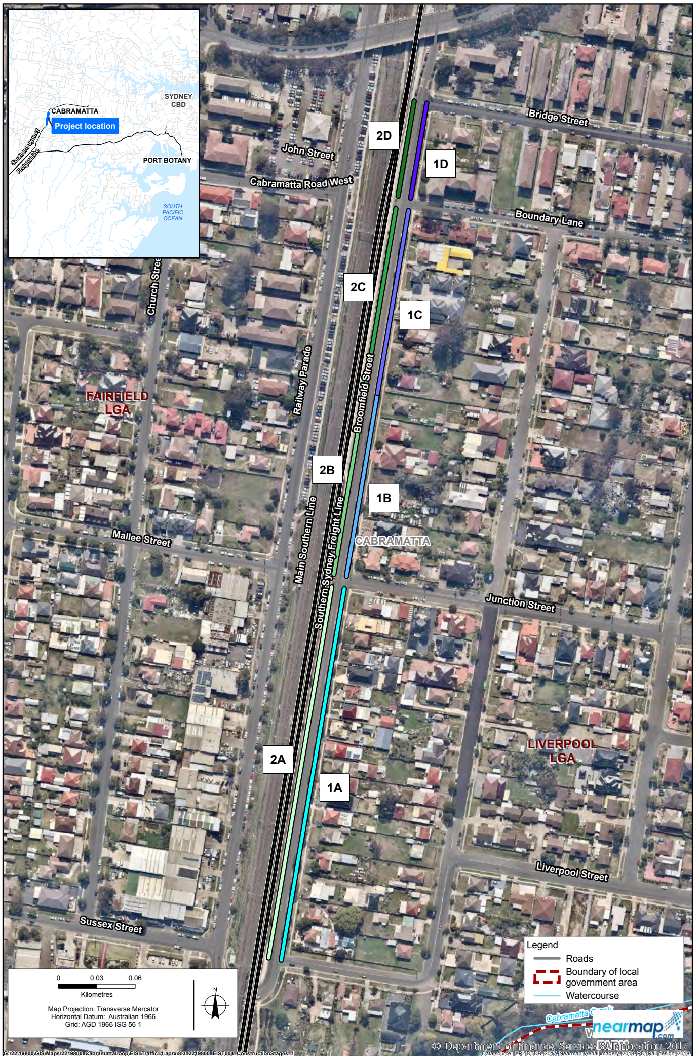
Figure 8.3 Construction stages along Broomfield Street
