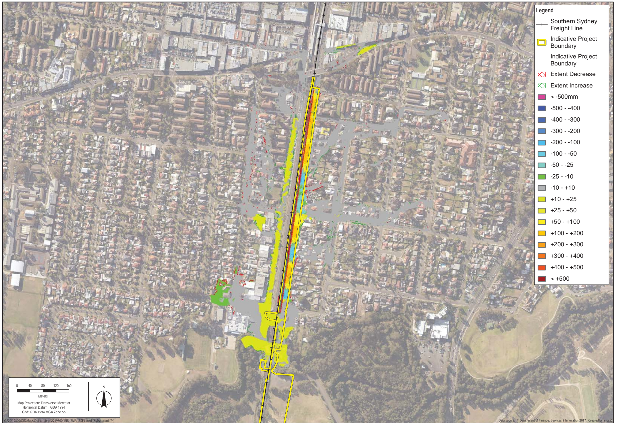
Figure 13.8 - Change in flood depth and extent with the project (Broomfield Street drainage only)– one per cent AEP
