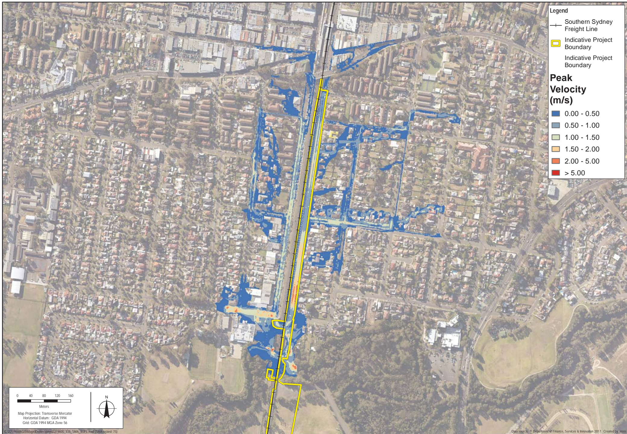
Figure 13.9 – Change in flood velocity with the project (Broomfield Street drainage only)– one per cent AEP
