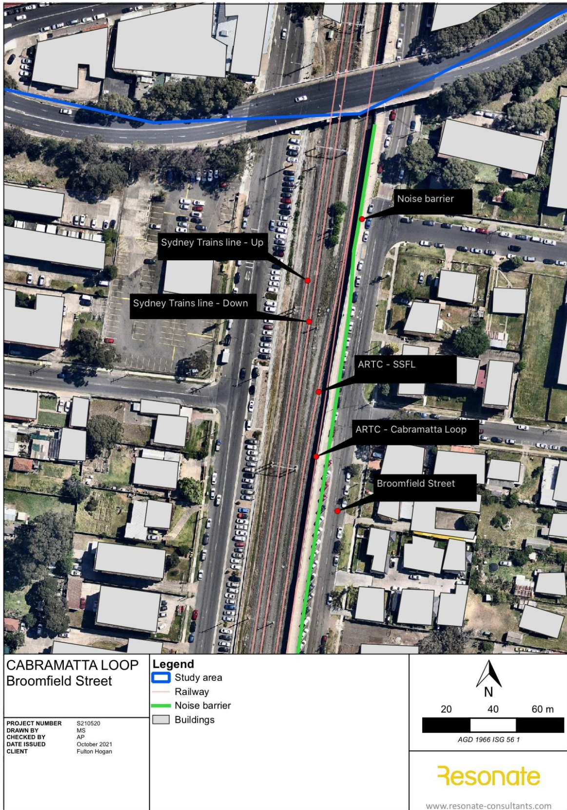
Figure 4: Noise barrier location along Broomfield Street
