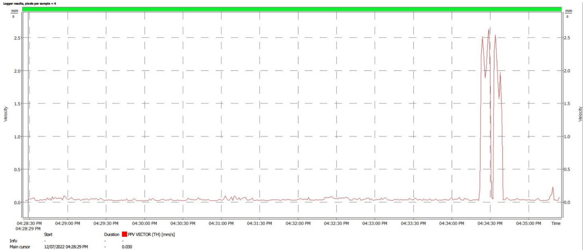
Above: Monitoring results from 170 Broomfield Street on the 12 th July 2022. Vibration peaked at 2.5mm/s.
