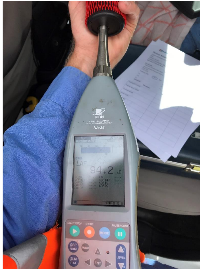
Above: Calibrating the machine at 94 dB(A) before monitoring in December 2022.
