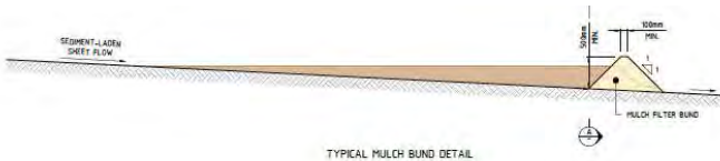
TYPICAL MULCH BUND DETAIL SCALE 1:50
