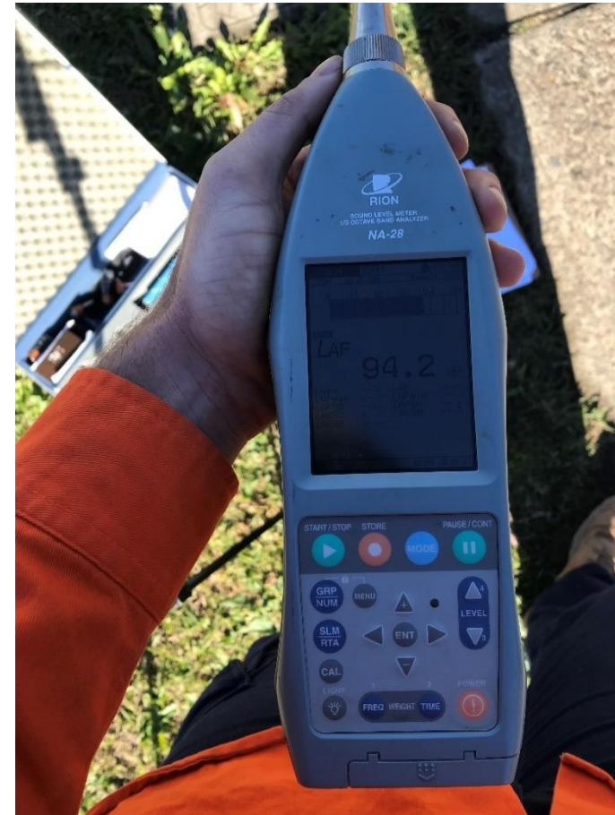
Above: Calibrating the machine at 94 dB(A) before monitoring in June 2023.
