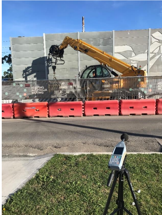
Above: Attended monitoring at 150 Broomfield St (NML2) during noise panel relocation works in May 2023.
